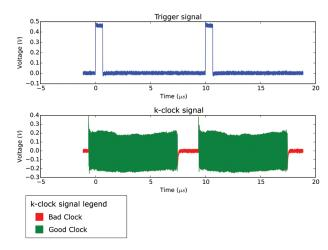
Users must set the trigger source to be External Trigger input (TRIG IN) when using OCT Ignore Bad Clock. The External Trigger must be set in TTL input range. If these two conditions are not met, the OCT Ignore Bad Clock circuitry will not function.
