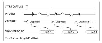
Continuous AutoDMA buffers do not include headers, so it is not possible to get trigger time-stamps. A BUFFER\_OVERFLOW flag is asserted only if the entire on-board memory is used up.
