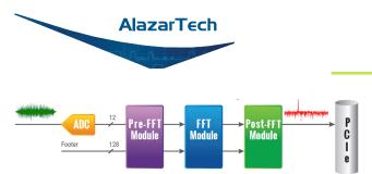
The complex FFT output is converted to magnitude in single precision floating-point format. A logarithmic output is also available.
