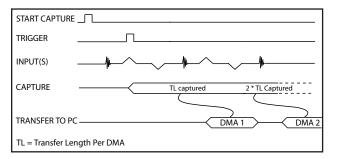
Triggered Streaming AutoDMA can easily acquire data to PC host memory at the maximum sustained transfer rate of the motherboard without causing an overflow. This is the recommended mode for RF signal recording that has to be started at a specific time, e.g. based on a GPS pulse.
