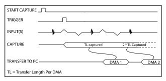
Triggered Streaming AutoDMA can easily acquire data to PC host memory at the maximum sustained transfer rate of the motherboard without causing an overflow. This is the recommended mode for RF signal recording that has to be started at a specific time, e.g. based on a GPS pulse.
