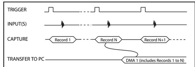
Note that a DMA is not started until (RecordsPerBuffer + 1) number of records (triggers) have been acquired and written to the on-board memory.
