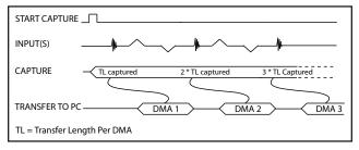
Continuous AutoDMA buffers do not include headers, so it is not possible to get trigger time-stamps.
