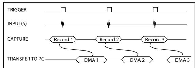
Data is returned to the user in buffers, where each buffer can contain from 1 to 8191 records (triggers). This number is called RecordsPerBuffer.
