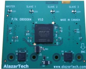
SyncBoard-9625 is available as a 2x or a 4x model: the 2x model allows a 2-board Master/Slave system whereas the 4x model allows 2, 3 or 4 board Master/Slave systems.
