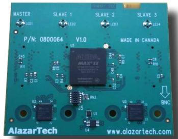
SyncBoard-9416 is a mezzanine board that connects to the Master/Slave connector along the top edge of the ATS9416 and sits parallel to the motherboard. For additional robustness, users can secure the SyncBoard-9416 to a bracket mounted on each of the ATS9416 boards.
