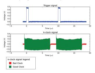
Firmware version 21.01+, driver version 5.10.6+ and SDK 7.1.3+ are required to take advantage of OCT Ignore Bad Clock. For existing customers, these firmware and driver versions are available for download from AlazarTech's website free of charge.
