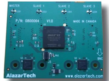
The Master board's clock and trigger signals are copied by the SyncBoard-9351 and supplied to all the Slave boards. This guarantees complete synchronization between the Master board and all Slave boards.
