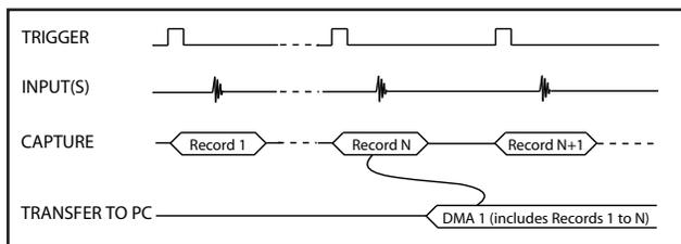
Note that a DMA is not started until RecordsPerBuffer number of records (triggers) have been acquired.
